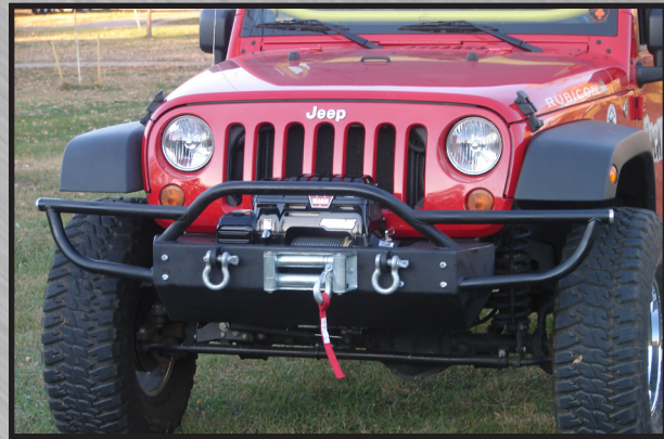
SHORTY FRONT BUMPER JK WRANGLER WITH TUBE EXTENSIONS LOWERED WINCH PLATE & 2 LIGHT TABS NO FOG LIGHT CUTOUTS
