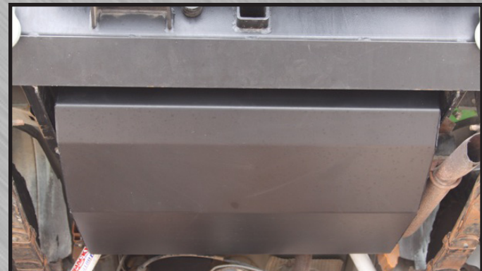
XJ CHEROKEE 1984-2001 FUEL TANK SKID MADE OF 3/16" STEEL PLATE CNC LASER CUT & BENT POWDER COATED BLACK FITS 2 & 4 DOOR
