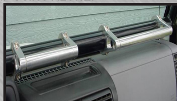
GRAB HANDLES FOR 1 3/4" TUBING CLAMPS ONTO CAGE - BILLET ALUMINUM 12" LONG PART #RH1020L $79.95 EACH 6" LONG PART #RH1020S $79.95 EACH
