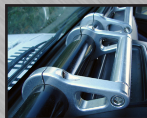
GRAB HANDLES FOR 1 3/4" TUBING CLAMPS ONTO CAGE BILLET ALUMINUM $79.95 EACH 12" LONG #RH1020L 6" LONG #RH1020S
